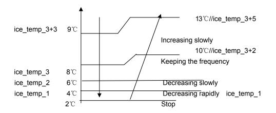
When Tpg\_indoor  $\langle$  ice\_temp\_1, the frequency of the compressor decreases at the speed of 1HZ/1second.
