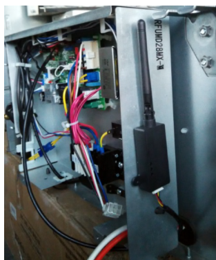
Installation Location Diagram of IDU Wireless Module
