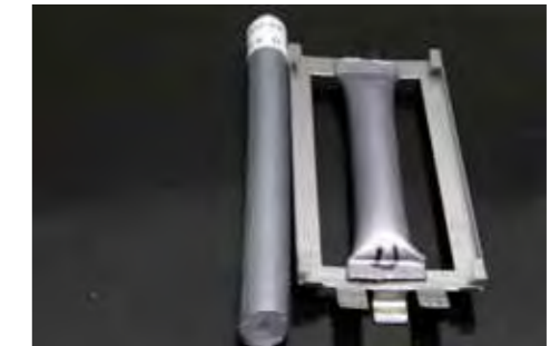
Zero hour sample (prior to exposure) and a sample subjected to an accelerated ageing test after 4000 hours of exposure.
