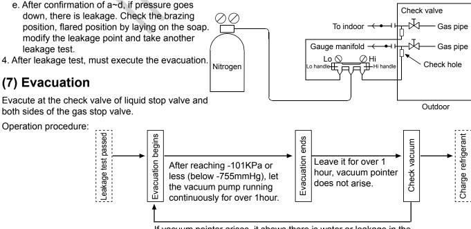
If vacuum pointer arises, it shows there is water or leakage in the system, please check and modify it, and then evacuate again.
