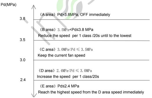
All the heating start, after the 4-way valve reversing (including defrosting, oil return and 4-way valve is electrified) the fan motor speed refer to the following:
