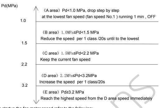
When startup the fan motor speed refer to the following:
