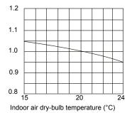
C. Capacity modification value under airflow variation rate of indoor unit group (only for duct unit)
