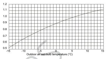
D. Capacity compensation suitable for total capability of indoor unit group
