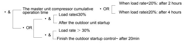
Note: load rate=∑indoor HP(Thermo ON) / ∑indoor HP\*100%
