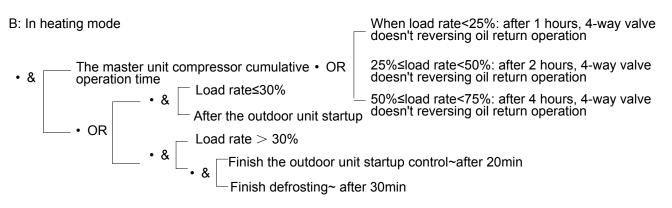
Note: if load rate≥75% and the outdoor unit output rate≥75% for 10 min, oil return time reset
